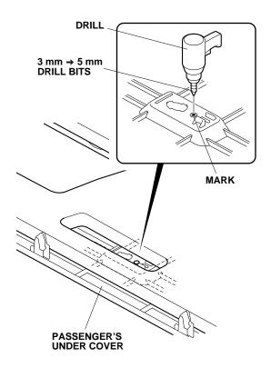
35. Install the ambient light to the passenger's under cover with one 4 x 12 mm self-tapping screw.
