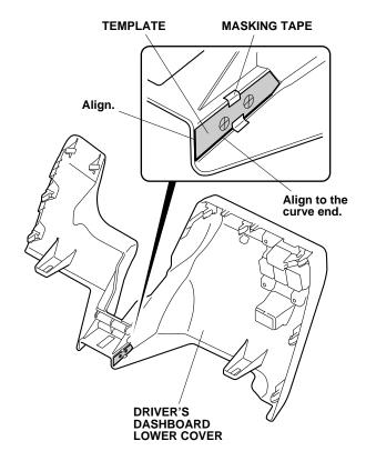
27. Using a pushpin, pierce the center of the two marks on the template.
