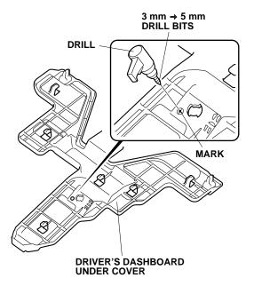
23. Install the ambient light to the driver's dashboard under cover with one 4 x 12 mm self-tapping screw.
