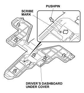
22. While wearing eye protection, drill the pierced mark on the driver's dashboard under cover with a 3 mm drill bit, then enlarge the hole to 5 mm using a 5 mm drill bit. Remove all burrs.
