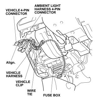
Align the ambient light harness 4-pin connector with the vehicle 4-pin connector, and secure the ambient light harness to the vehicle harness with one wire tie. 8. Plug the vehicle 4-pin connector into the ambient light harness 4-pin connector.
