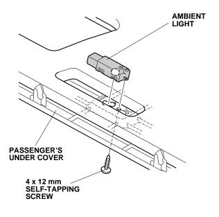
36. Plug the ambient light harness 4-pin connector into the ambient light, and reinstall the passenger's under cover.
