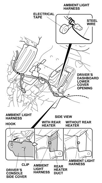
14. Attach a piece of steel wire to the ambient light harness with electrical tape. Route the ambient light harness through the center console from the driver's dashboard lower cover opening to the passenger's under cover opening. 15. Release the passenger's console side cover (two clips).
