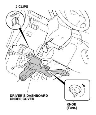
Remove the driver's dashboard lower cover (nine clips and unplug the vehicle connectors).
