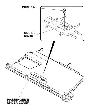
34. While wearing eye protection, drill the pierced mark on the passenger's under cover with a 3 mm drill bit, then enlarge the hole to 5 mm using a 5 mm drill bit. Remove all burrs.
