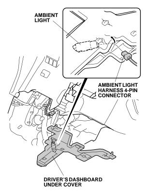
38. Plug the ambient light harness 4-pin connector into the ambient light, and reinstall the driver's dashboard under cover. Go to step 40.
